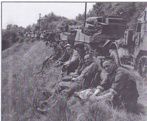
During a halt, crews eat a quick meal. Exhaust adapters can be seen on the rear of most of the tanks wading chutes tied onto the engine decks. The tank in the centre of the photo is a Firefly with its turret reversed to point at 7-o'clock. Closest to the camera is an M5 or M9 Halftrack, each Squadron had one of these
