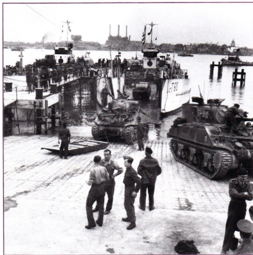
More tanks loading onto LCTG/O. Note the amphibious jeep just entering the craft. The tank that will follow it tows a Porpoise, its towing bars are tied to the hull front
